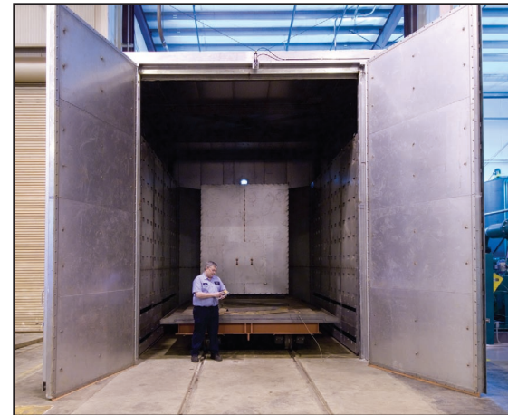
Bakeout Oven used to cure VPI epoxy resin
